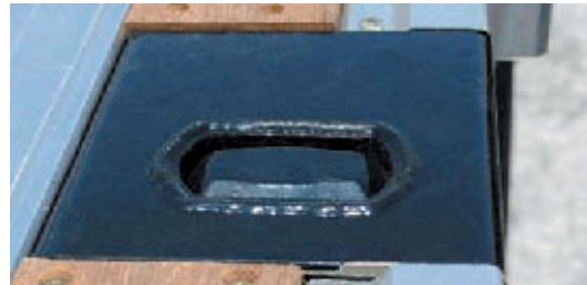
■ Twist Locks can be incorporated into the design for securement of containers atop the flatbed.
