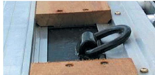
■ D Rings are recessed below the floor level.
