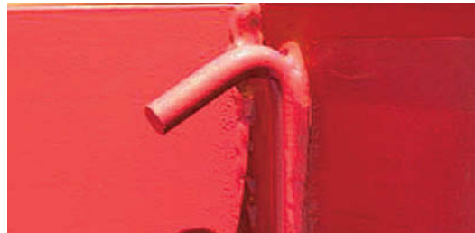
■ Rope Ties are welded to the side rail or under side of the trailer between crossmembers.
