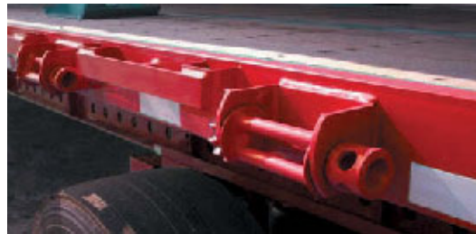
■ 3-Bar Winches make load securement fast and easy.
